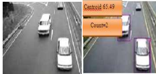
Fig.3. Tracking of moving objects and its count using background subtraction method
